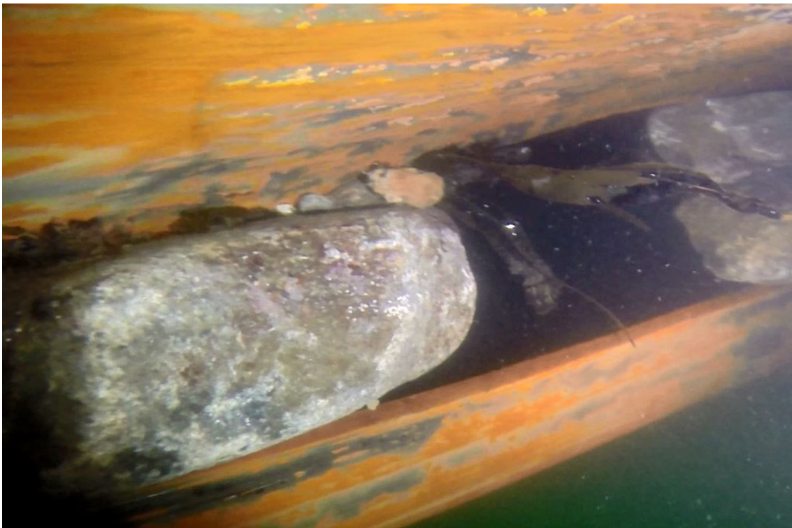
Figure 18: Damage to the starboard side hull. Source: Peter Doehle Schifffahrts-KG/DMAIB
