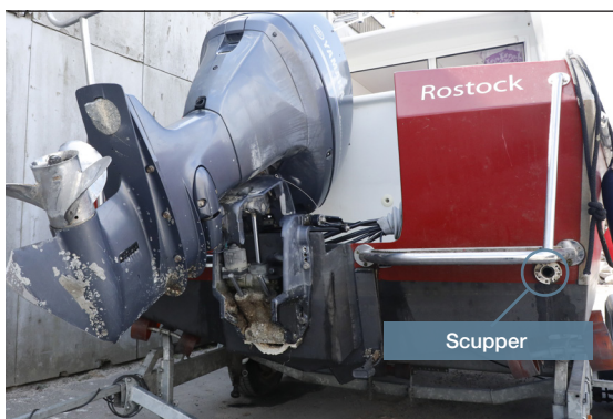
Figure 16: Self-bailing arrangement. Note the absence of non-return flaps on the scuppers outside. Source: DMAIB
