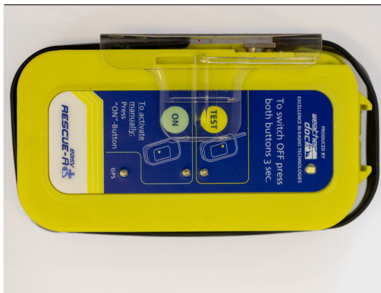
Figure 25: AIS-SART attached to Secumar lifejacket Source: DMAIB
